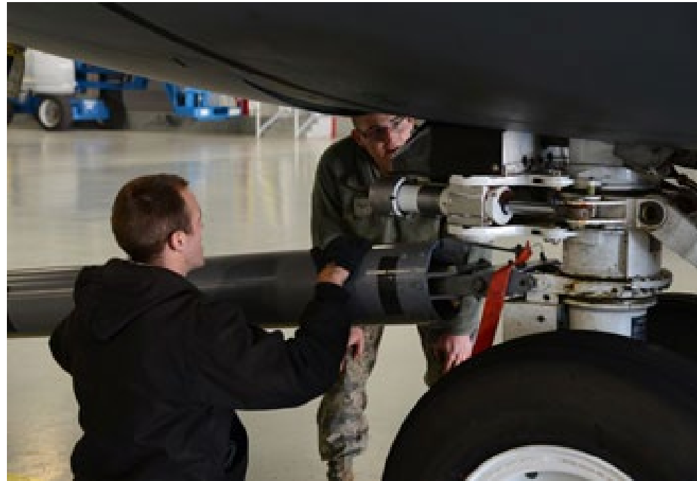
Master Sgt. Robert Ahern, a 137th Air Refueling Wing crew chief, left, and Airman 1st Class Mykal Short, a 507th Air Refueling Wing ISO Dock crew chief, hook up a tow bar and make sure the sheer pin is installed to be able to tow a KC-135 Stratotanker to the trim pad for engine runs. The 137th ARW, an Oklahoma Air National Guard unit, is a partner unit with the 507th ARW. The Airmen of both units work side-by-side to ensure the planes are well-maintained for mission capability. (Air Force photo by Kelly White)
